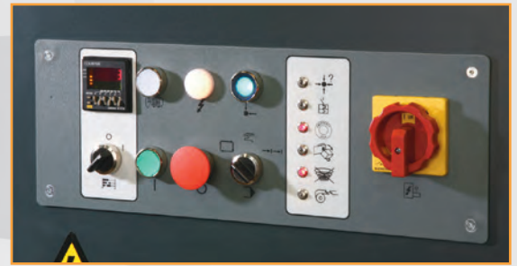
Control panel with visual indicators of operation anomalies
