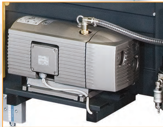
Vacuum pump for box picking
